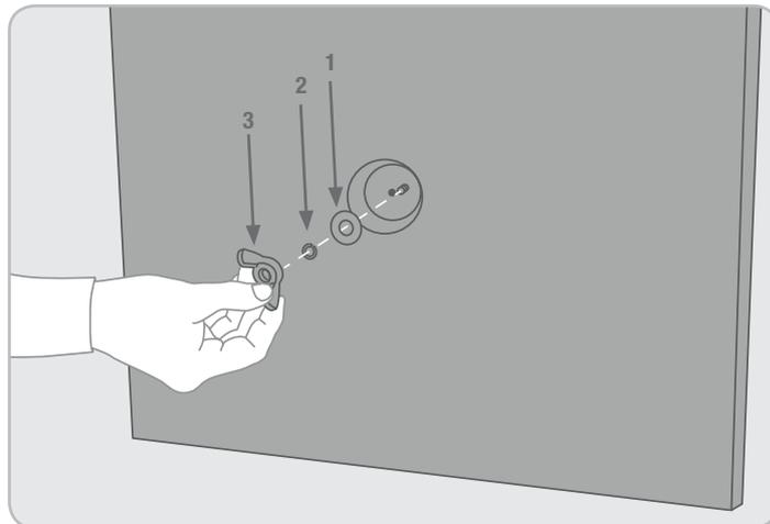
**6** First place the repair washer, then the spring washer & finally the wing nut onto the exposed threaded pin & hand tighten until the flat plate on the post fits snugly against the rubber base.
