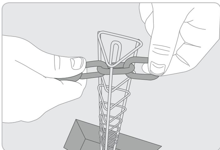
**7** Thread the first link on the chain through the top section of the upright and position onto the integrated hook. Continue by feeding the opposing end of the chain through the adjacent upright until the sag in the chain is approximately 100 mm below the horizontal then attach the intermediate link to the hook.
