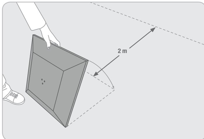
**2** Measure 2 m from the hazard whilst being sure to stay at a safe distance from the edge. Remaining within the safe zone, position the first base at this point, placing it down outwards, away from the body as shown, with the D-marc logo facing away from the hazard.
