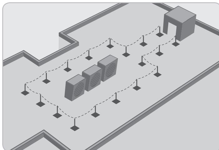
**8** Thread the rest of the chain through the D-marc 105 uprights until reaching the final upright, where the remainder of the chain should be trimmed using tin snips. Should multiple lengths of chain be required join each by using the split chain link supplied.
