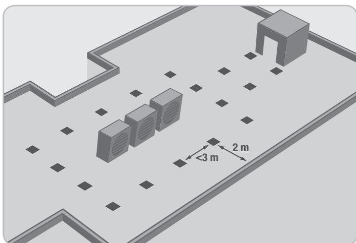
**3** Lay the rest of the bases in the same way along the edge of the demarcation zone at regular distances of no more than 3 m apart. Should a corner post be required the bases may be positioned at 90° degrees from each other or even at an acute angle.
