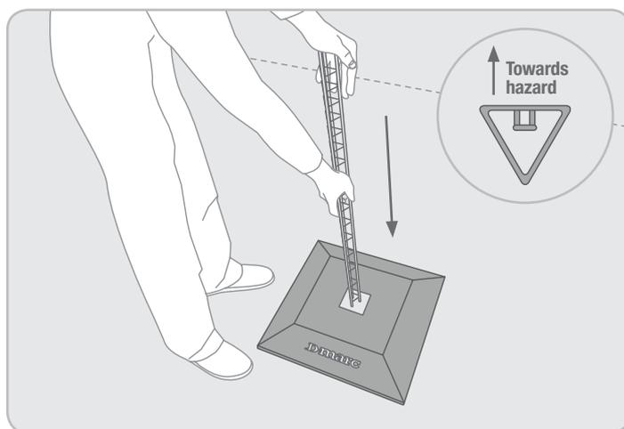
**4** Insert the D-marc 105 upright into base ensuring the integrated hook for the chain is on the side facing the hazard. The upright base plate must fit flush into the weighted base.
